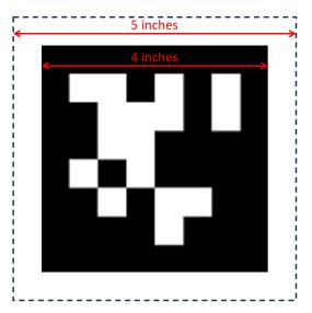
Figure 1: Dimensions for a 4-inch 36h11 AprilTag
